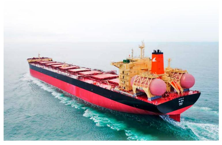
In 2020, Panama flagged the world's first LNG-powered bulk carriers, HL Green and HL ECO operated by H-Line Shipping. The vessels have a cargo capacity of 180,000 DWT and are 292 m length overall, 45 m breadth moulded and 18.0 m draught.
